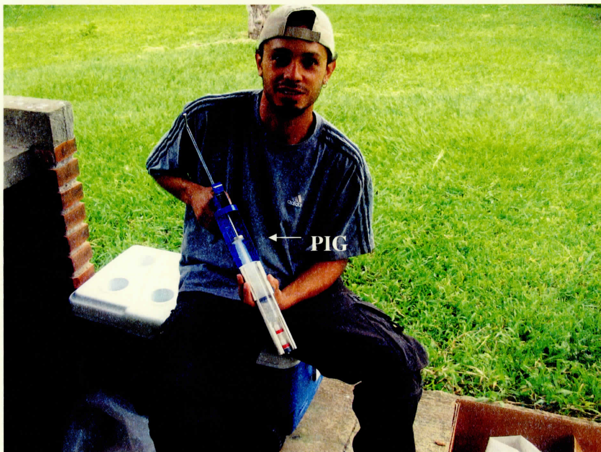
Figure 5. Peptide Injection Gun (PIG). New tool addition to the peptide extraction methodology, used to force fluids through the SepPak cartridges with 50ml syringes.
