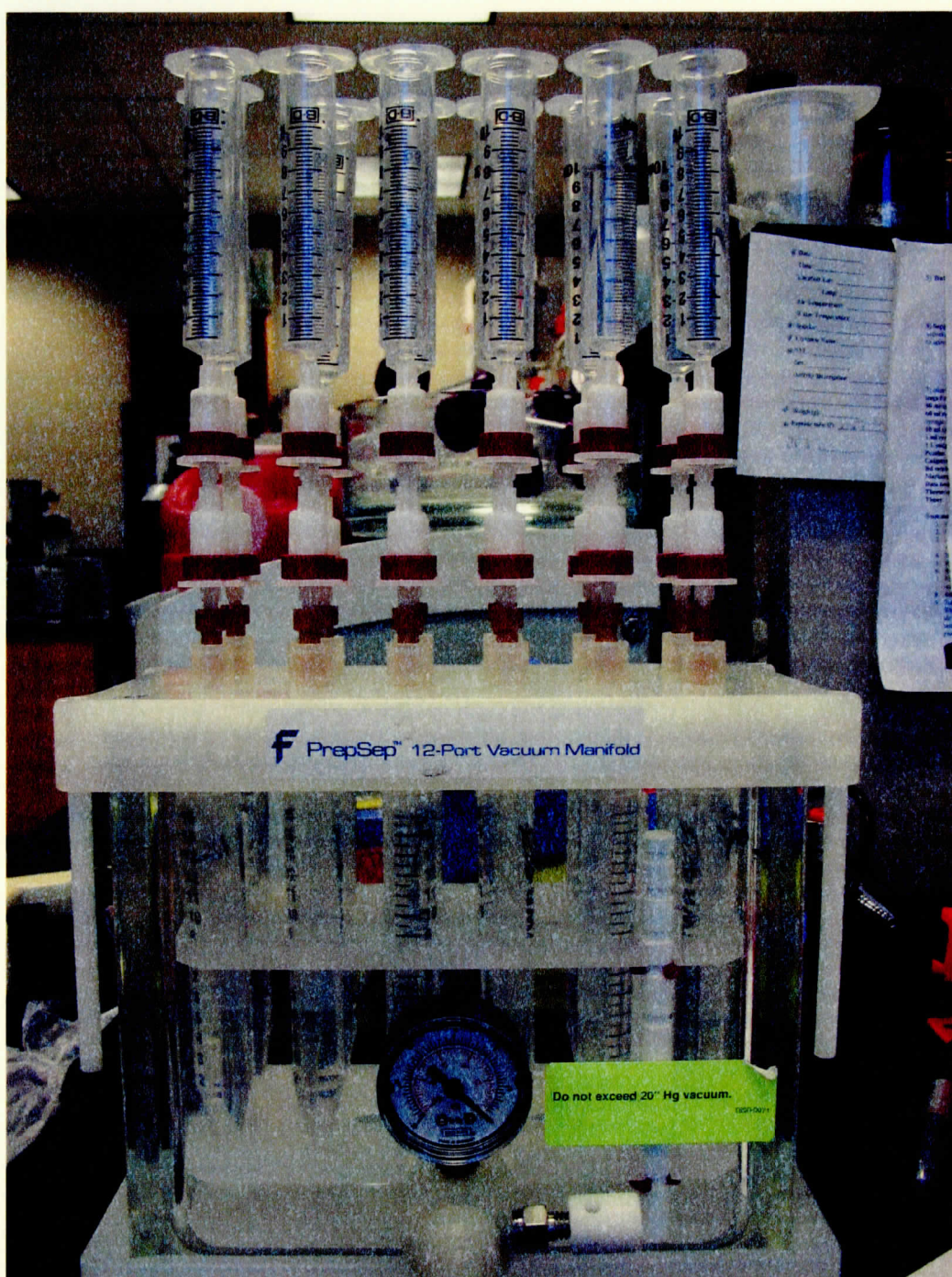
Figure 6. PrepSep 12 port Vacuum Manifold. Pressure vacuum used to extract the peptides from the SepPak cartridges and SepPak cartridge activation.
